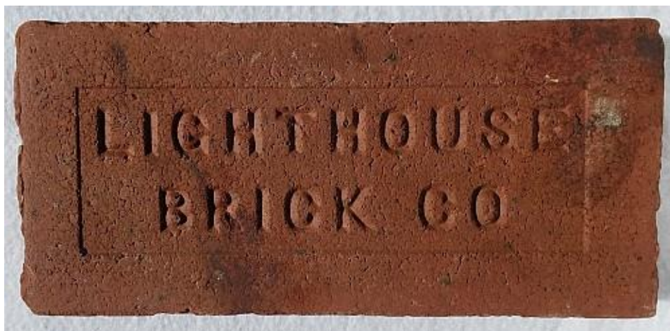
Fig 49. Dry Pressed brick by Lighthouse Brick Co, 1933-1939.
