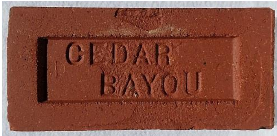
Fig 50. Dry Pressed brick from John Kilgore's yard, 1939-1958.
