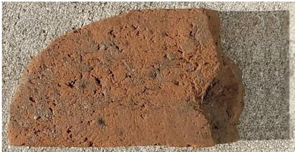
Fig 35. Molded curb brick from Casey & Gillette brickyard, ca 1904.
