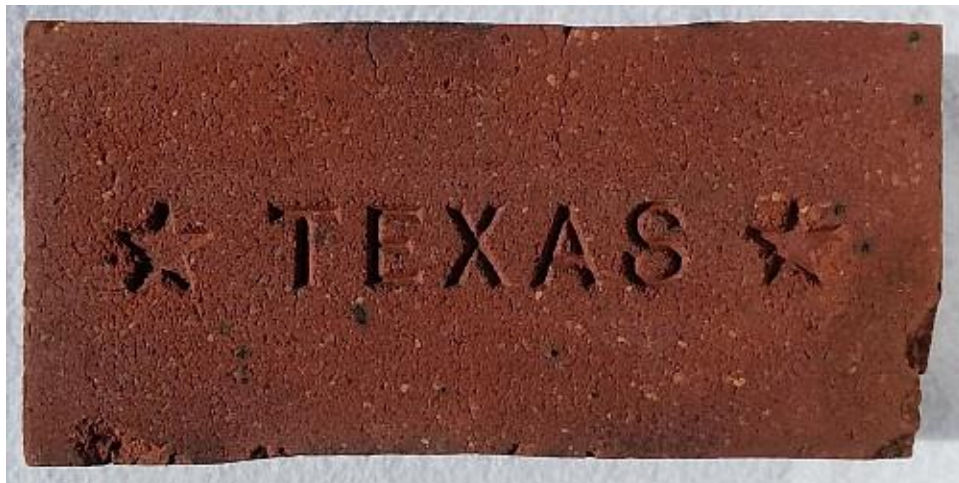
Fig 47. Dry pressed brick by Texas Brick & Tile Co, 1927-1928.
