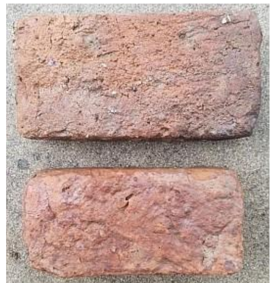
Fig 59. Bricks from Thomas Edgar’s yard. He made two sizes of brick. The larger brick is entirely handmade as evidenced by the diagonal striations and un-pressed folds in the clay. The bottom is a very weathered machine made brick.
