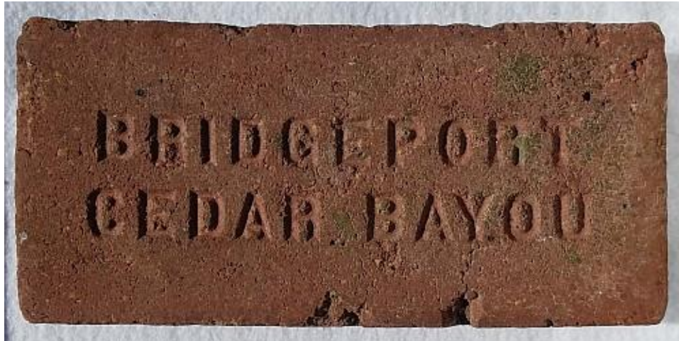
Fig 48. Dry Pressed brick by Bridgeport Brick & Tile Co, 1928-1930.
